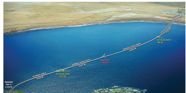
The 36 km long causeway will connect Kuwait City (bottom of the photo) and Shubiyah New Town.
