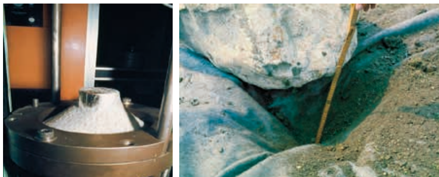
Figure 6.4 Static puncture resistance (CBR test) compared to real-life installations
