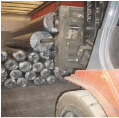
Figure 8.1 Unloading the rolls using a forklift mounted with a spear
